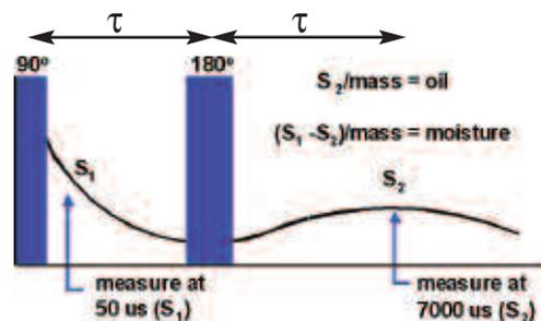
The oil and moisture signal is measured from the FID and the oil signal from the echo. The moisture signal is obtained by taking the difference between these two values.
